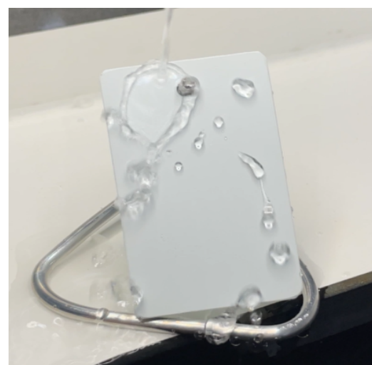
Figure (b) super hydrophobicity on Cirrus Lustre™ Surface
